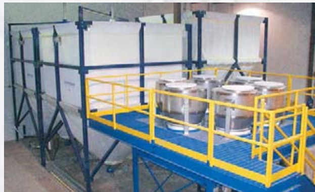
▲ A four station multi-ingredient system for accurate metering of yeast, sugar, flour and baking soda
